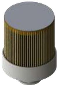
Star filter elements with a large surface are built into each adsorber. This ensures that the total pressure build-up of the adsorber is not caused by the filter.
