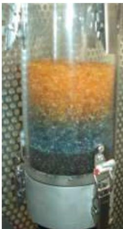
In the course of using an adsorber, the silica gel is loaded with water molecules, i.e. the free surface in the pores is filled. This reduces the binding energies for further absorption.
