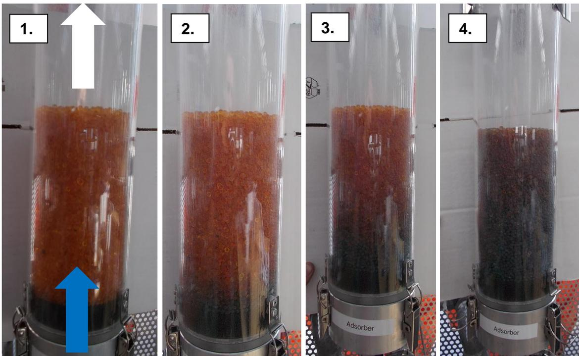
Figure 1: Color gradient of an adsorber with 1.5 kg of silica gel with increasing loading.
