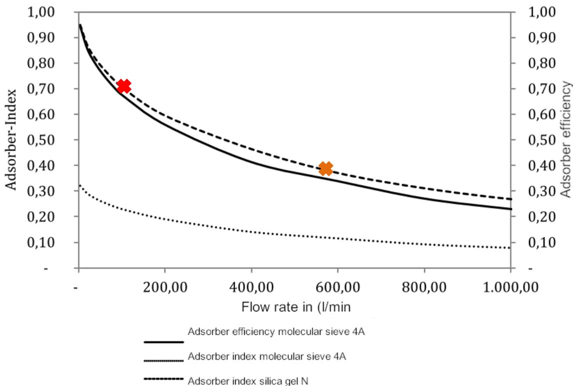
Figure 2: Adsorber index at 20 ° C and an adsorber with 1 kg desiccant mass, depending on the volume flow.
