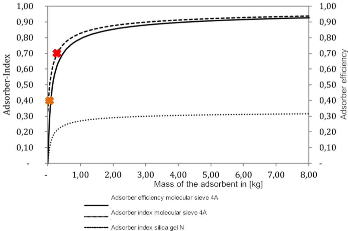
Figure 3: Adsorber index at 20 ° C at a flow rate of 40 l / min, depending on the dry matter mass.
