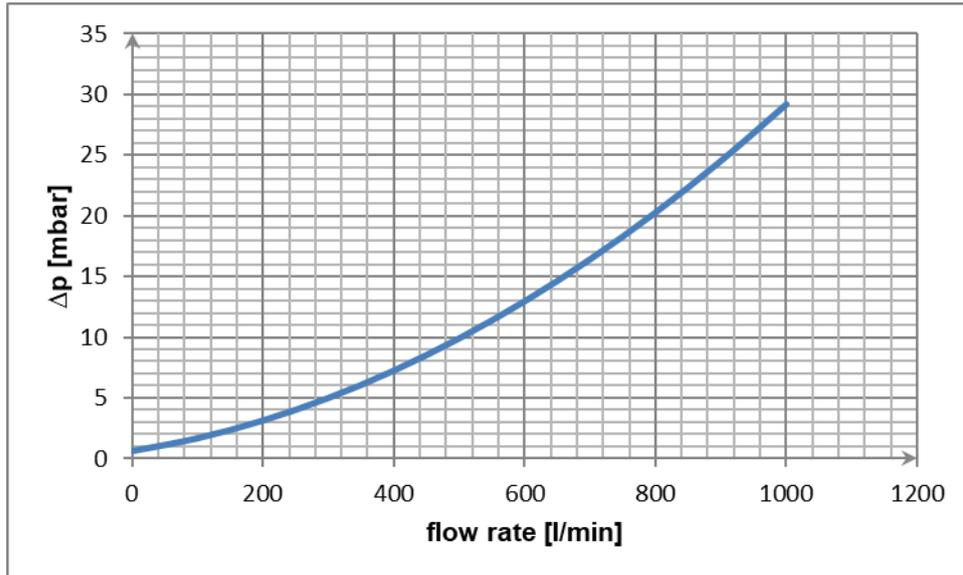
Figure 4: Pressure difference of an adsorber (without valves), depending on the volume flow.
