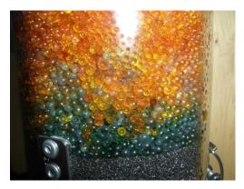
**4. Adsober, or the desiccant are oiled.** Silica gel loaded with oil has lost the ability to adsorb water. The pores are impregnated and therefore closed. The color change takes place only partially, with a considerable delay and with a different color.
