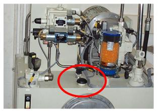
**3.** Air does not flow through the adsorber. If there is an opening in the system through which the air can be drawn in, it is not dried. The air thus bypasses the adsorber. This does not absorb water and remains new for a longer period.
