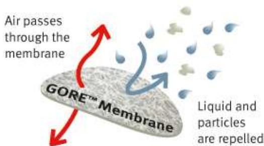
Figure 2: Function of the hydrophobic GORE membrane. (see [www.gore.com](http://www.gore.com))
