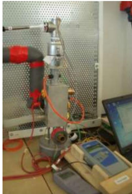
Figure 3: Test setup for the separation of air humidity.
