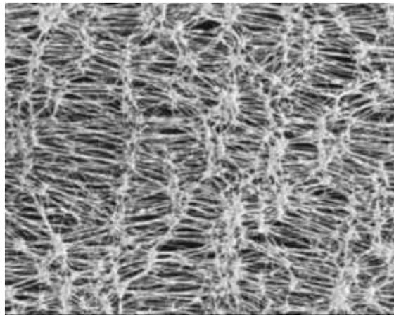
Figure 1: Electron micrograph of an ePTFE structure.
