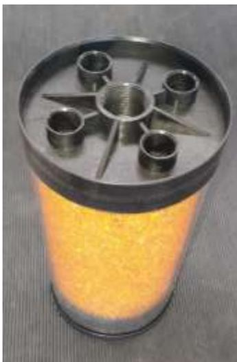
1. Adsorber after filling and bonding.
