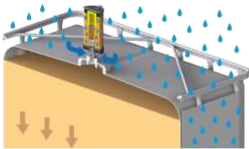
The determination of the maintenance interval for the ventilation of drums and IBC containers depends on the container. For example, an adsorber is screwed onto a drum. As soon as it is completely emptied, the drum ventilation filter is mounted on a new, full drum. With this change, an air volume of 200 l or 1000 l is.
